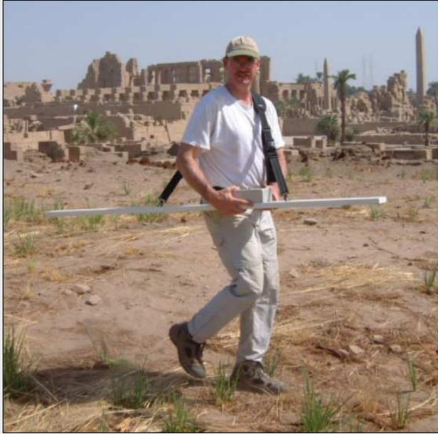
Typical Geopex EM unit used to define Pirate Tunnels
